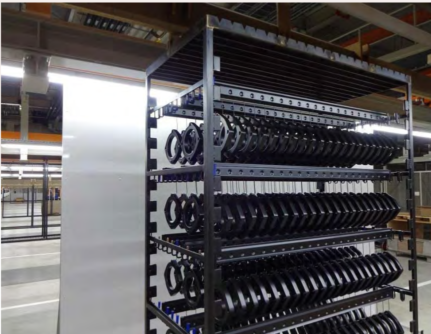
Universal KTL immersion box with several mounting levels for flexible equipment. The component to be coated is picked up in a crossbar by means of hooks. This works on the principle of a dipping bell, so that the contact points always remain free of paint.
