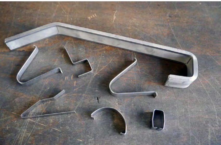
Spring clips made of VA spring steel and suspension hooks made of flat material (30 x 8 mm).
