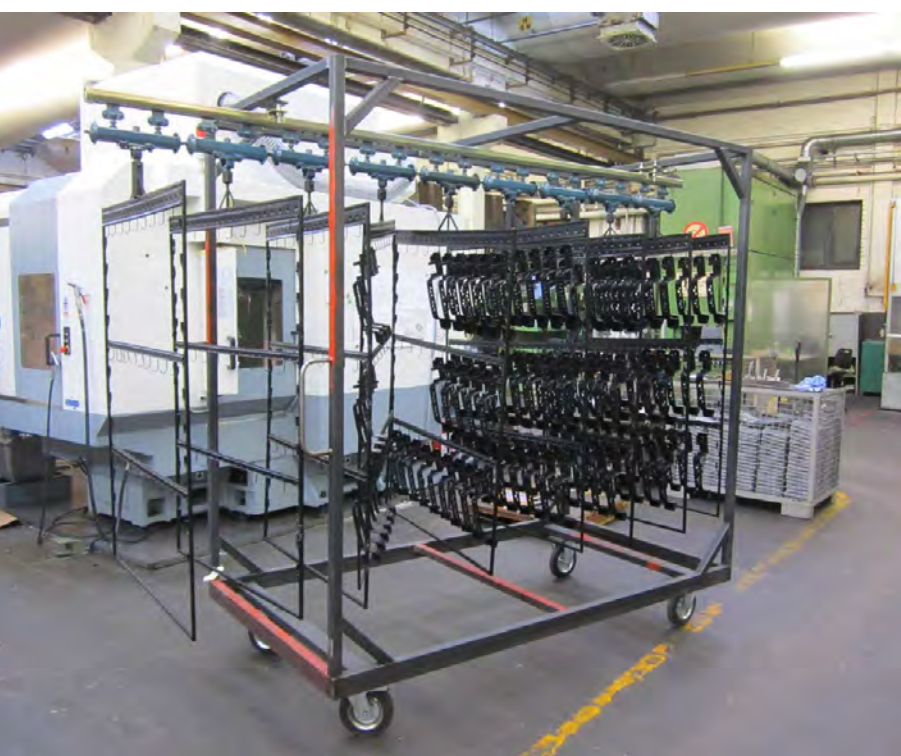
Preloading trolley for metal matrix racks including trolley for quick transfer to the painting line.
